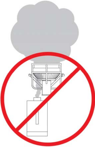
Incorrect ProFan placement in front of fogger/hazer
